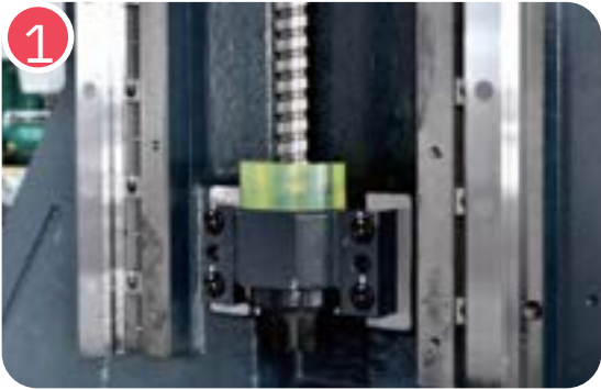
The Z-axis uses a new pre-tensioned structure which can suppress the thermal expansion of the lead screw and offset the thermal expansion of the spindle, further enhancing the stability of the Z-axis precision.
