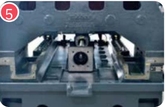
The columns use a large-span truss box structure Processing efficiency is stable
