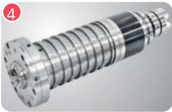
The spindle uses vibration-absorbing materials Effectively improving precision, and uses imported ceramic ball bearings, which provide high operational accuracy and low temperature rise. The short and thick pull stud make better rigidity and stronger cutting performance
