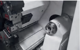
Programmable Tailstock It's applicable for bars of different lengths, stable precision, strong operability, simplicity, flexibility and superior rigidity are ensured.
